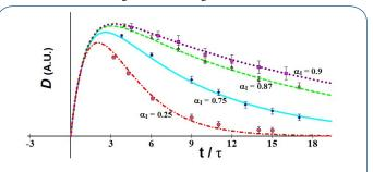
**Figure 1:** Diffusion behaviour vs time for some values of  $\alpha_I$  (see text) as prediction of the model. Dots are experimental data from THz spectroscopy [23], with distribution represented by error bars
