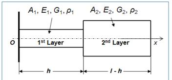
**Figure 1:** A sketch of the cantilever with one mechanical and geometric discontinuity
