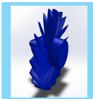
Figure 8: Mechanical drawing of Aero-Engine fan according to dimensions calculated in the present design by using solid-works software
