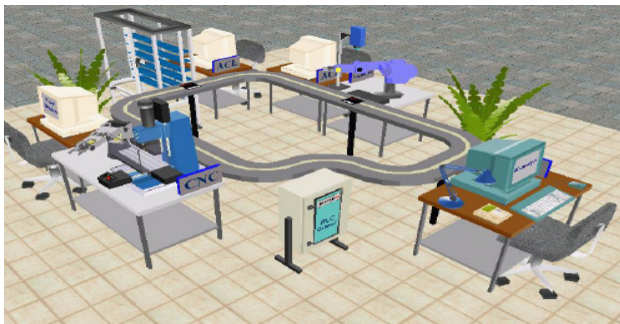
Figure 3: Graphic representation of a CIM system with three workstations
